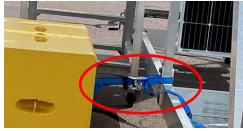
When using the GSE tie-down blocks, the operator is responsible in selecting an appropriate tether/strap to secure the equipment.
