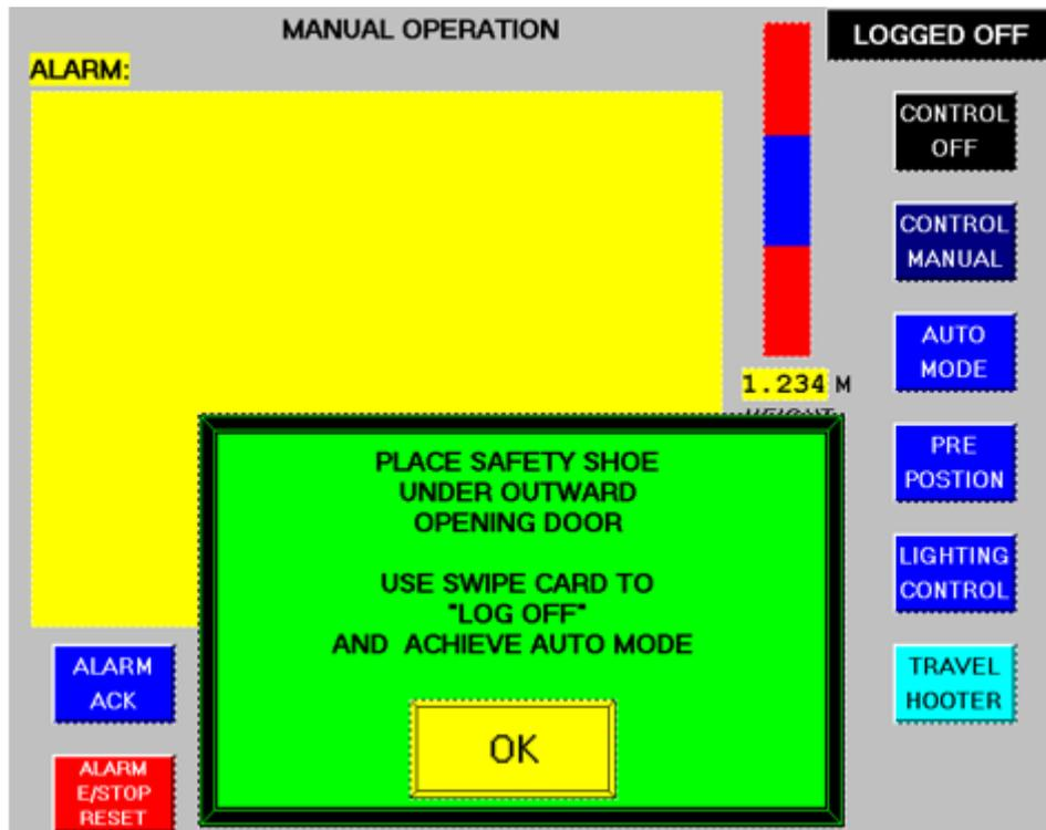
With the Aerobridge docked and in “AUTO” mode, the operator must log off with their swipe card.
